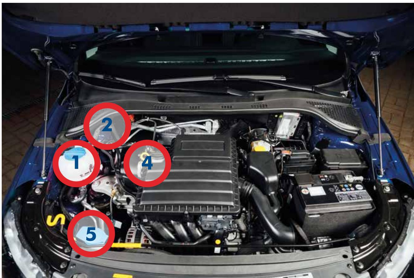
2] Open the bonnet, identify where the brake fluid reservoir is; how do you check you have a safe level of hydraulic fluid?
